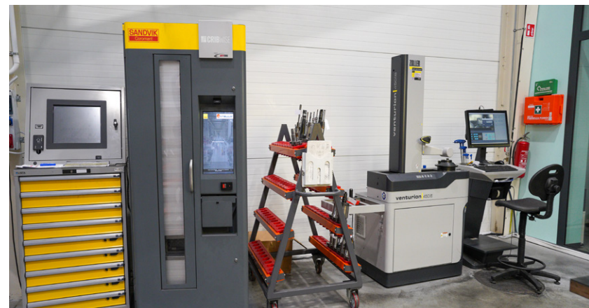
The tools are measured automatically using the Zoller automatic CNC scanner. Tool room equipped with automatic tool dispensing machines.
