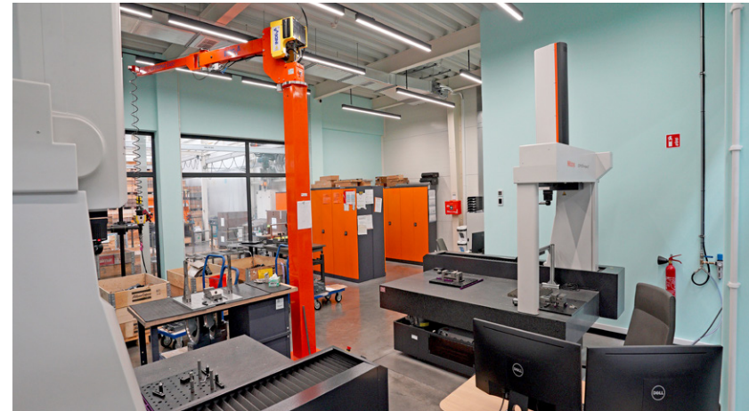
The measurement department is equipped with 2 automatic CMM coordinate measuring machines of Mitutoyo and GOM measuring scanner.
